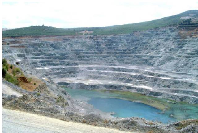
Fig. 3. Asbestos mine excavation using the open pit method.
